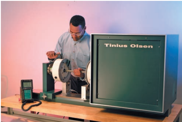
Photo 3.3 Tabletop torsion testing machine.
