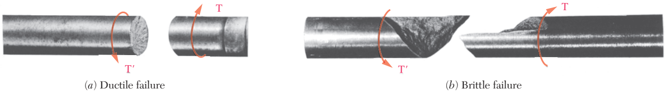
Photo 3.2 Shear failure of shaft subject to torque.
